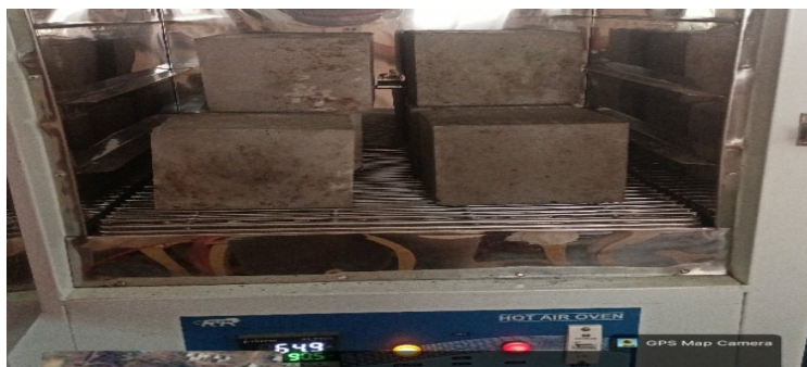
Fig 4 Heat Curing in Oven (90°C)
