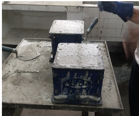
Fig 3 Concrete Cube Casting
